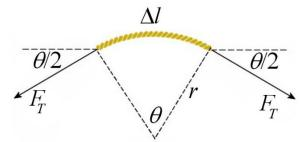
The tension forces and the angles being the same on each side of the piece, the sum of the x-component of the forces vanishes by symmetry. On the other hand, the y-components of the forces do not cancel out. The sum of these components is
