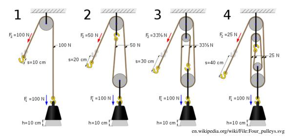
With the pulley system 2, the rope must be pulled 20 cm to lift the mass 10 cm. This is so because the rope supports the object attached to the pulley twice and it is necessary to reduce the length of the rope twice by 10 cm to lift the mass 10 cm. By multiplying the rope distance to be pulled by 2, the force is divided by 2.
