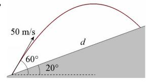
37. An object is launched on a slope, as shown on the diagram. Show that to reach the greatest distance on the slope, one must have
