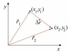
The displacement  $\overrightarrow{\Delta r}$ , i.e. the change in position, is a vector going from position 1 to position 2.
