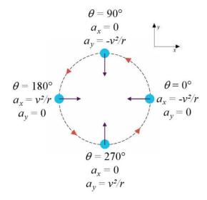
It is obvious that the acceleration is always  $v^2/r$  and is always directed towards the centre of the circle. This acceleration is called the *centripetal acceleration*, where *centripetal* means "towards the centre". This acceleration is denoted  $a_c$ .
