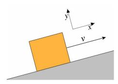
However, the axes must sometimes be rotated. Actually, there is only one restriction: the two axes must be perpendicular. For example, the axes shown on this diagram will be used for an object travelling along an incline (we will see in chapter 4 that an axis pointing in the direction of the velocity or in a direction opposite to the velocity must be used for a moving object).
