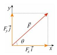
The components can easily be found with trigonometric functions.
