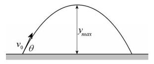
As  $y_0 = 0$  was used, the maximum height given by this formula is always measured from the starting point of the projectile. Solving for the maximum height, the result is
