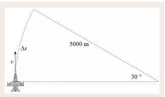
a) What is the distance travelled by the plane at this instant ( $\Delta s$  on the diagram)?
