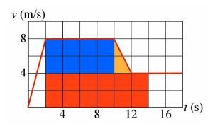
The area of the red rectangle is  $4 \text{ m/s} \times 12 \text{ s} = 48 \text{ m}$ .
