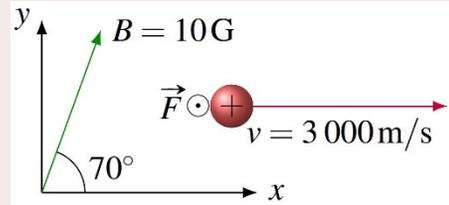
$$\begin{aligned} \vec{F} &= q\vec{v} \times \vec{B} \\ &= q \cdot \begin{vmatrix} \vec{i} & \vec{j} & \vec{k} \\ v_x & v_y & v_z \\ B_x & B_y & B_z \end{vmatrix} \end{aligned}$$
