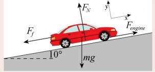
Since the car is moving at the same speed as it was on the horizontal surface, the frictional force is the same (402.8 N). The equation now becomes
