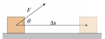
The unit used to measure work is the Nm. Another name was given to this unit: the joule (J).
