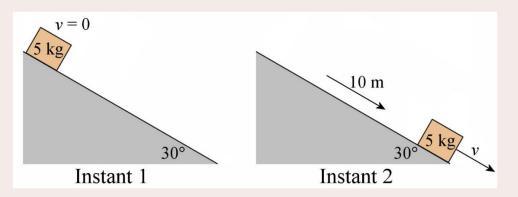
The work-energy theorem will be applied here for the motion between these two instants:
