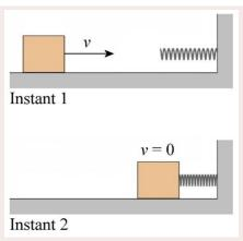
At instant 1, the spring is not compressed. Therefore, x = 0 m.
