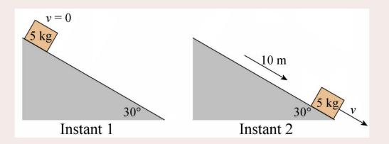
To find the work done by the forces, the forces acting on the box must be found first. There are 3 forces acting on the 5 kg box.
