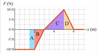
To find the work, the area under the curve between x = 1.5 m and x = 6 m must be calculated. To calculate this area, the area will be split into 4 regions (identified by the letters A, B, C and D on the graph).
